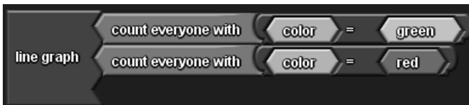
Fig. 6.20 Code to set up a line graph that tracks the number of green and red agents.
