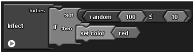
Fig. 6.10 Infect Run Once code to seed the infection at the start of the simulation.
