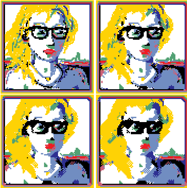
Fig. 8.25 Top Left: A 2D seed, n = 88 \times 88 , drawn with the mouse and keyboard, [v, k] = [8, 4] . Colors 0 to (v - 1) can be selected. The image/seed can be moved, rotated, and complimented. Sub-patterns saved earlier can be loaded into specified positions within the main pattern. In this example the seed is then transformed by applying a CA majority rule for three time-steps.
