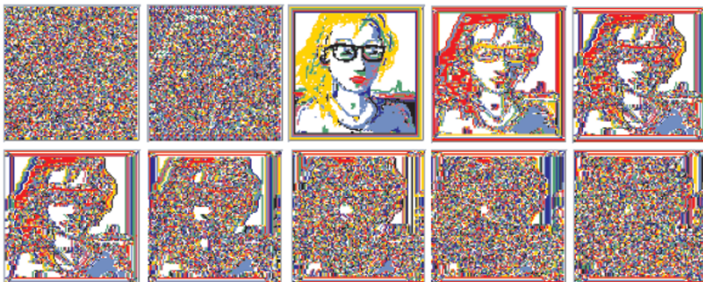
Fig. 8.43 To decrypt, starting from the encrypted state in Fig. 8.42, the CA with the same chain-rule was run forward to recover the original image. This figure shows time-steps -2 to +7 , to illustrate how the portrait was scrambled both before and after time-step 4.
