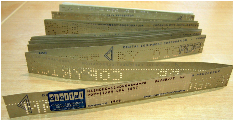
Figure 8.6 A fanfold DEC paper tape containing a PDP-11 test program. (Reproduced by permission under the GNU Free Documentation License, photographer: Unknown, source: http://en.wikipedia.org/wiki/Image:Papertape2.jpg )
