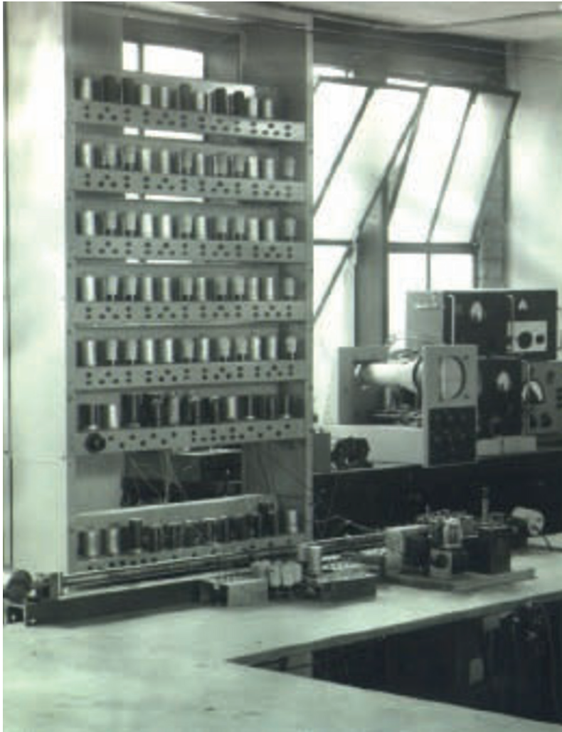
Figure 8.4 Experimental EDSAC memory tank. (Copyright Computer Laboratory, University of Cambridge. Reproduced by permission under the Creative Commons Attribution Licence, photographer: Unknown, source: http://www.cl.cam.ac.uk/Relics/jpegs/edsac99.23.jpg )
