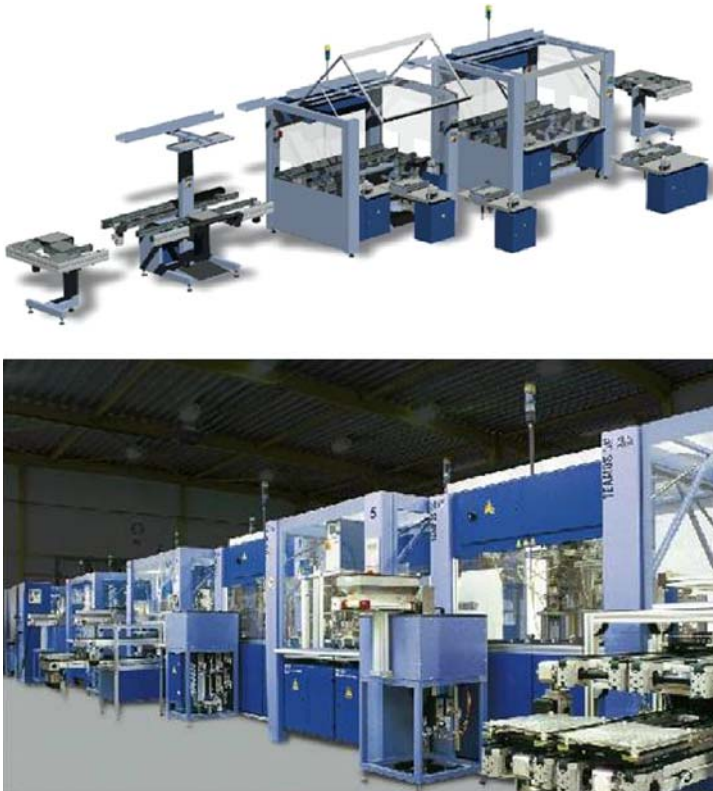
Fig. 4.3 Reconfigurable system “Teamos” for assembly and finishing operations [team-technik, Germany]
