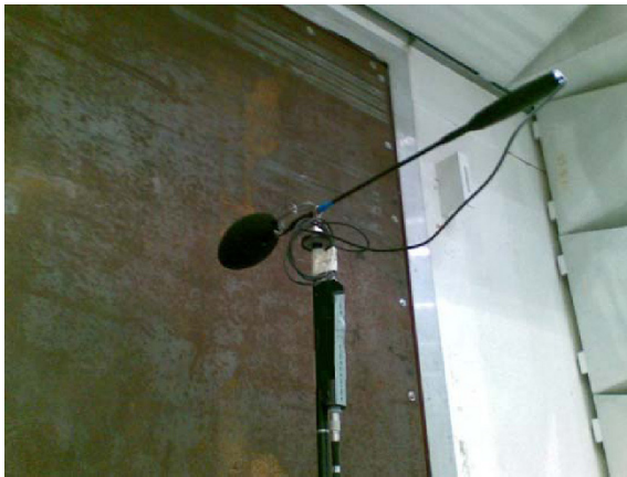
Figure 5. Intensity probe used for the ISO 15186 tests
