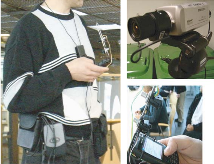
Fig. 4 Version 2 of Fig. 1's mobile video recording system. Some characteristics: (a) All noncamera equipment except cables fit on a belt and weigh less than 2 kg in total; (b) Feed from the closest environmental camera is integrated into the four-video recording. (c) All video and audio inputs are integrated on the fly to a four-video display; (d) The cameras are flexible, can be worn or attached to the mobile device, and can operate with cables or wirelessly; (e) There is an option for remotely triggered recording events initiated via Bluetooth; (f) Operational duration is up to 4 hours without battery change or other maintenance operations
