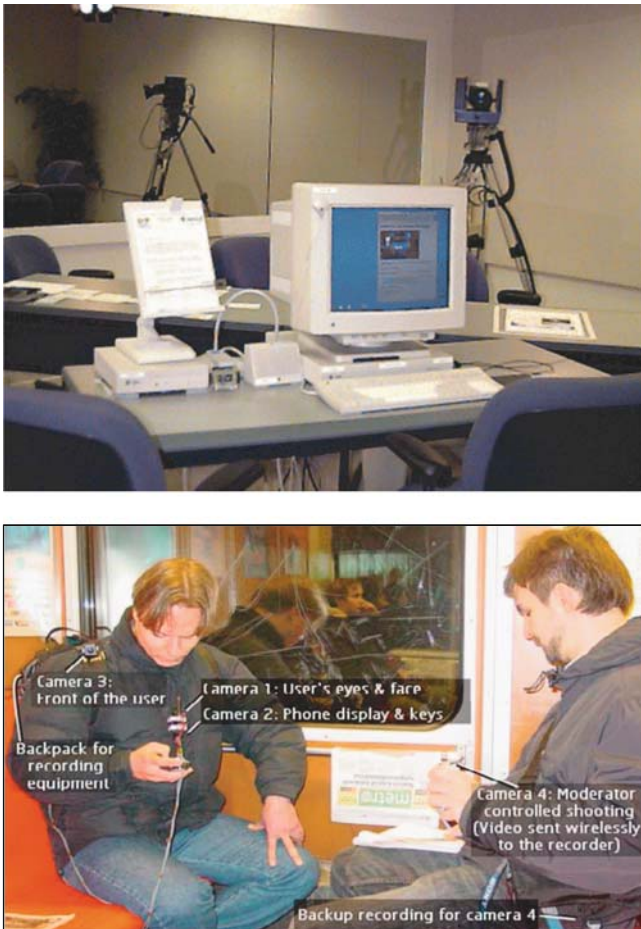
Fig. 1 Two setups for experimentation in HCI. On the top , Jakob Nielsen’s (1995) laboratory setup at Sun Microsystems that worked as a model and baseline for many laboratories built around the world in the 1990s. On the bottom , one of the first published “mobile usability labs,” developed in joint effort between Nokia Research Center and HIIT (Roto et al., 2004)
