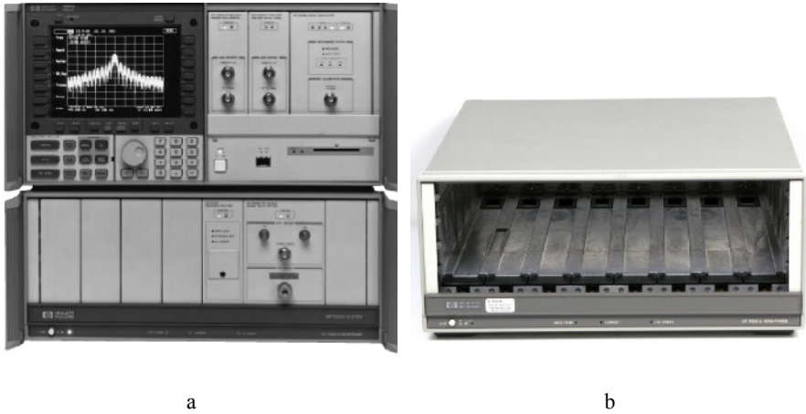
Figure 6.17. HP 70000 series spectrum analyzer: a modular system; b mainframe power (courtesy of Hewlett Packard)
