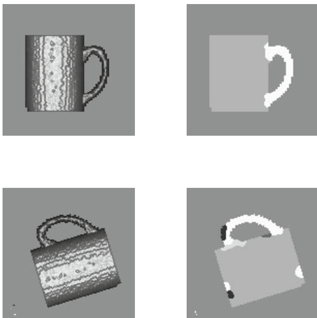
Figure 4.3: Cup images and segmentation based on H - K surface curvatures. Top: A cup image and its H - K map. Bottom: A transformed version of the cup image and the H - K map (note that some noise is introduced after the transformation due to quantization). From (Li 1992c) with permission; ©1992 Elsevier.
