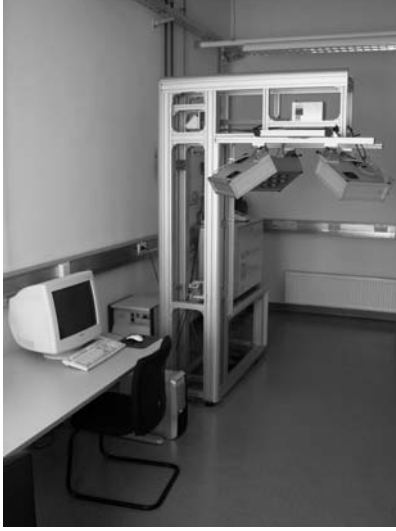
Figure 1: System technology of the sensor based automated excimer laser treatment system for inflammatory skin diseases like psoriasis
