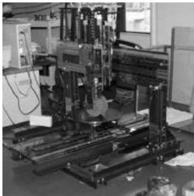
Figure 13: Machine tool for ISO 14649 CNC data model.
