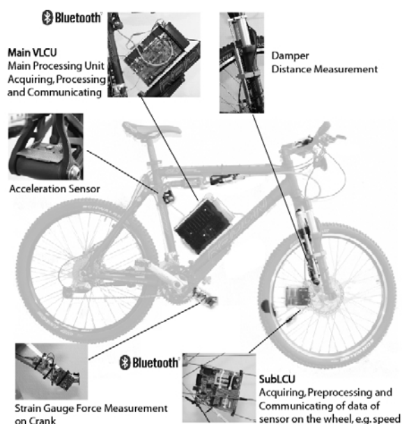
Figure 9: Conceptual VLCU application on a bicycle for use in a PSS business model.
