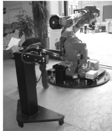
Figure 2. One of the mobile fixtures and one robot on a base-plate developed in demonstrator 1.
