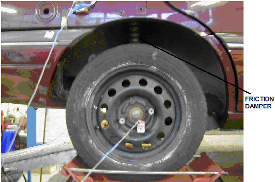
Fig. 7.15. Friction damper installed on the experimental vehicle
