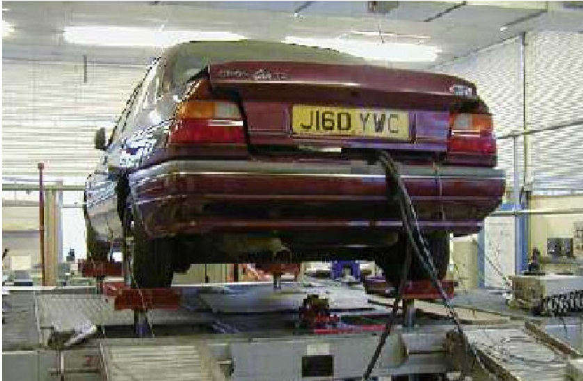
Fig. 7.1. Test vehicle on the four-poster road simulator
