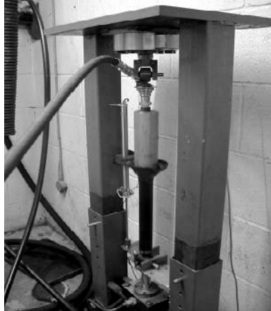
Fig. 5.17. Friction damper on the bench rig
