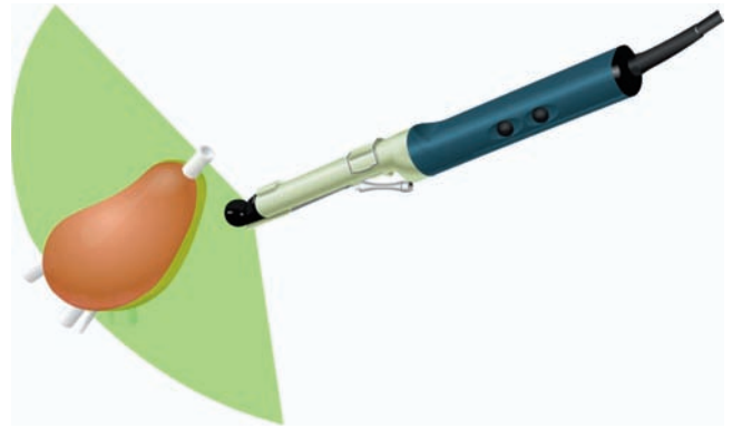
FIG. 11.20. Illustration of the scan plane when the transducer is used in endfire mode
