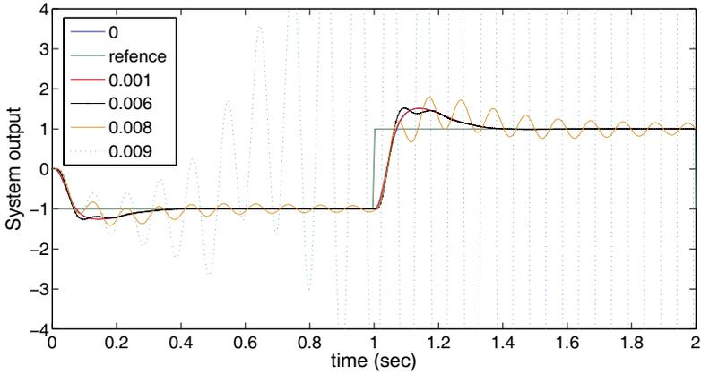
Fig. 8.5. System outputs under different fixed delays
