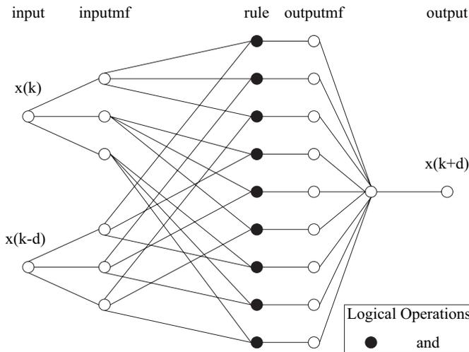
Fig. 8.12. The structure of the ANFIS predictor
