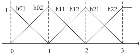
Fig. 8.6. The local fuzzy weighting functions of the example
