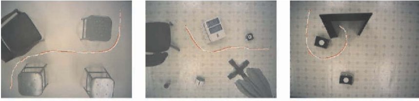
Fig. 1.17. Navigation results of the networked control navigation system for different environmental patterns. White line is the ideal path and dark line is the actual path traversed by the robot.
