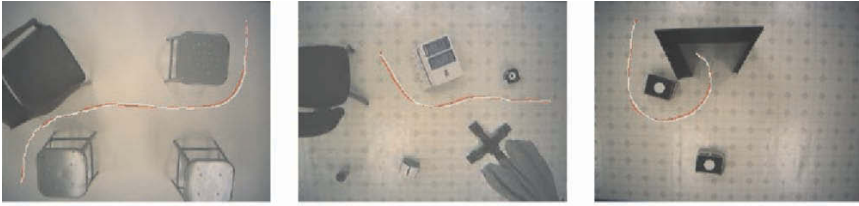
Fig. 1.17. Navigation results of the networked control navigation system for different environmental patterns. White line is the ideal path and dark line is the actual path traversed by the robot.
