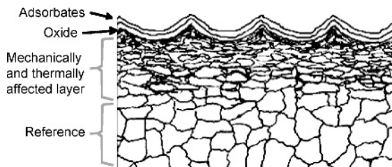
Figure 3.2. Schematic section of a machined surface
