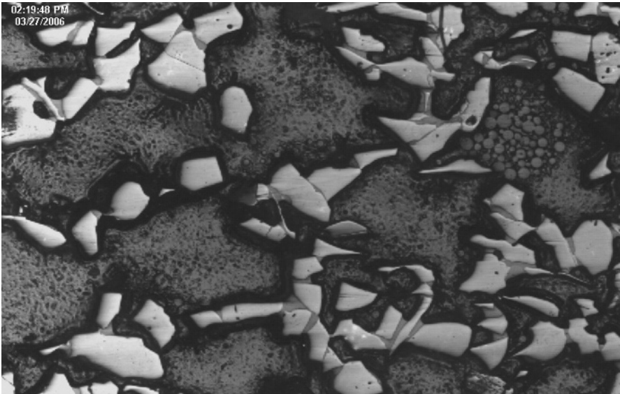
Figure 9.2. Micrograph of conventional grinding wheel with distributed porosity
