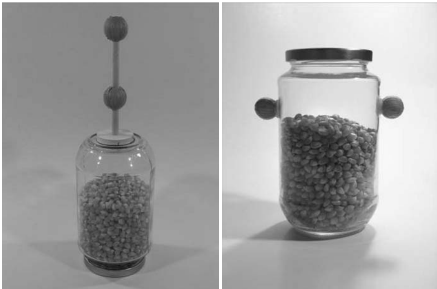
Figure 5.3. The jar on the left is a set up for subjects who place their hand on the side of the jar: the jar on the right is set up for subjects who place their hand on the bottom of the jar
