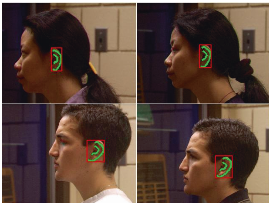
Fig. 3.24. Results of ear localization on the UND dataset shown in Figure 1.5. The helix and the anti-helix parts are marked by the bright dots and the detected ear is bounded by a rectangular box.
