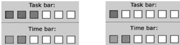
Figure 1. Left: the awareness display representing a timely interruption – the task bar is ahead of the time bar meaning that the Helper advances with the task and experiences low time–pressure; Right: the awareness display representing an untimely interruption – the time bar is ahead of the task bar meaning that the Helper stays behind the task and experiences high time–pressure.
