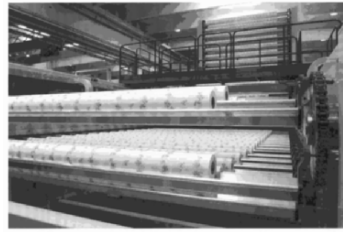
Figure 2: Unacceptable cast on paper rolls
