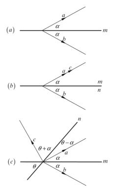
as the separating angle between the mirrors is  $0^\circ$ , the separating angle between *a* and its double reflection *c* is also  $0^\circ$ .
