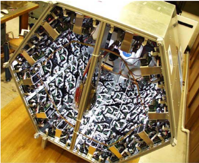
Fig. 4.1. The hexagonal prism physical implementation of the CD test-bed structure, lying on its side with the end open to reveal the cellular internal structure of the electronics.
