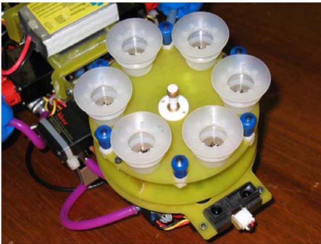
Fig. 4.8. The ultrasonic transducer mounted in the centre of the robot's foot.
