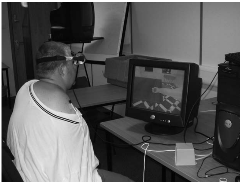
FIGURE 11.2. The Bournemouth phantom. A motion capture device is placed on the subject's right shoulder, which drives the movement of the virtual arm.
