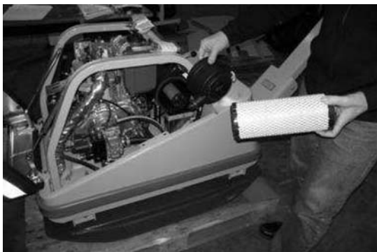
Figure 6: The adapted air filter in Swepac's soil compactor FB-455.
