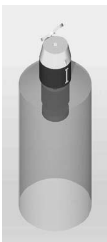
Figure 1. Schematic view of the double-dose liquid dispenser bottle top
