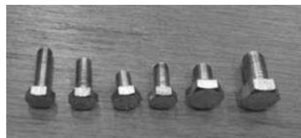
Figure 7b. Screws used in soil compactor FB-200H.
