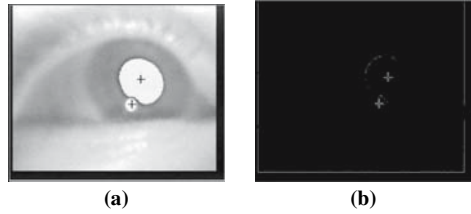
Fig. 4.2 (a) Original eye image from the eye tracker (left); (b) output of the Canny enhancer (right) distribution.
