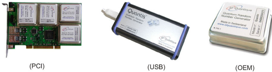
Fig. 13.3 idQuantique’s quantum random number generator [405] is available as a PCI board, a USB device, or as a component ready for mounting on a printed circuit board. It has been tested and certified by the Swiss Federal Office of Metrology. Images courtesy of idQuantique
