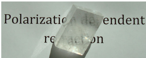
Fig. 13.4 How a birefringent crystal can be used to separate photons based on their polarization. In the figure shown, a naturally cleaved and unpolished calcite crystal is placed on top of the text “polarization dependent refraction” and illuminated with sunlight containing a mixture of polarizations. As a result reflected ordinary rays are refracted through the crystal via one path and reflected extraordinary rays are refracted by a slightly offset path. This causes the blurring of the letters that are visible through the crystal. We can therefore use where the light rays emerge from such a crystal to measure their polarization state
