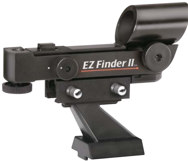
Figure 7.4. A unit-power (non-magnifying), reflex-sight finder like that now widely used on telescopes in place of (or in conjunction with) conventional optical finders. It works simply by superimposing a tiny LED red dot focused at infinity on a 10-degree view of the sky, showing exactly where the telescope is pointed. Courtesy of Orion Telescopes & Binoculars.
