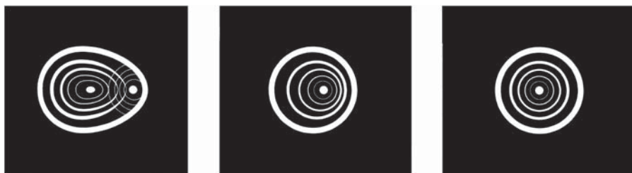
Figure 1.3. The out-of-focus (extrafocal) image of a star can reveal many things about a telescope's optics (as well as about its thermal environment and the state of the atmosphere) – in this case, the alignment of the optical components. The image in the left-hand panel reveals gross misalignment. That in the middle panel shows moderate misalignment (still enough to degrade image quality), while the image in the right-hand panel indicates perfectly collimated optics.
