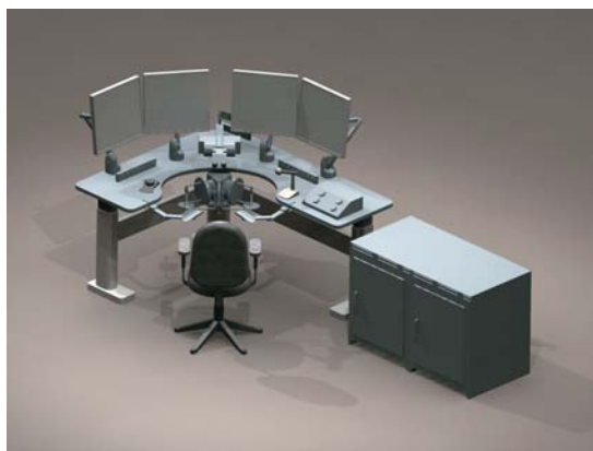
FIGURE 3.2. neuroArm workstation. (Reprinted with kind permission of Alexander Greer, Seaman Family MR Research Centre, Foothills Medical Centre, Canada.)
