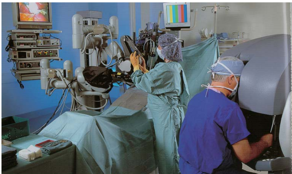
FIGURE 26.2. The computer console of the da Vinci® Surgical System radically extends the capability of the digitally integrated operating room. The console's computer can integrate the digital data from imaging systems such as CT and MRI scans into the
