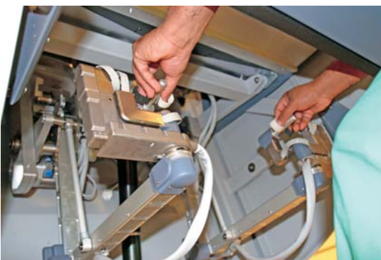
FIGURE 2.5. Surgeon's hands in the finger controls, which translate the finger and wrist movements into electrical signals.
