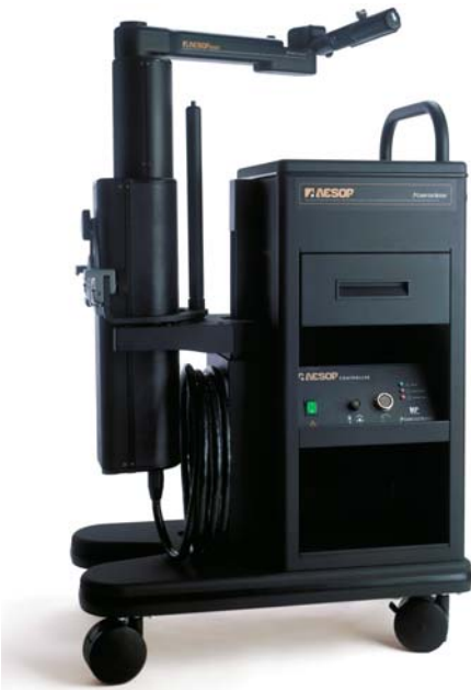
FIGURE 2.1. The AESOP system with robotic arm to hold the laparoscopic camera, which can be controlled by foot switch or voice control. (Reprinted with kind permission from Intuitive Surgical, Inc. www.davinciprostatectomy.com/images/aesop_images.zip and www.davinciprostatectomy.com/images/zeus_images.zip by Alexis Morgan, Sunnyvale, CA, USA. January 2007.)
