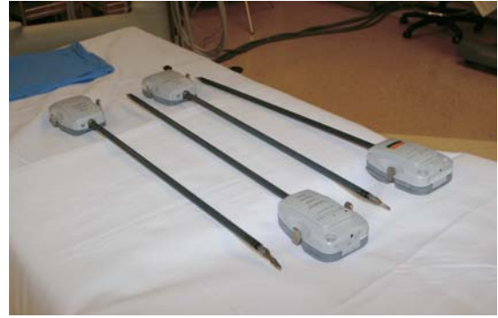
FIGURE 2.9. Different robotic instruments like dissectors, graspers, and scissors. The operational life of each instrument is roughly 10 cases.
