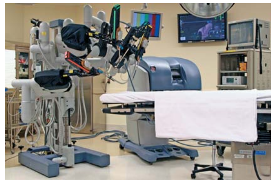
FIGURE 2.3. Three components of the da Vinci ® robotic system: console, surgical cart, and video cart.
