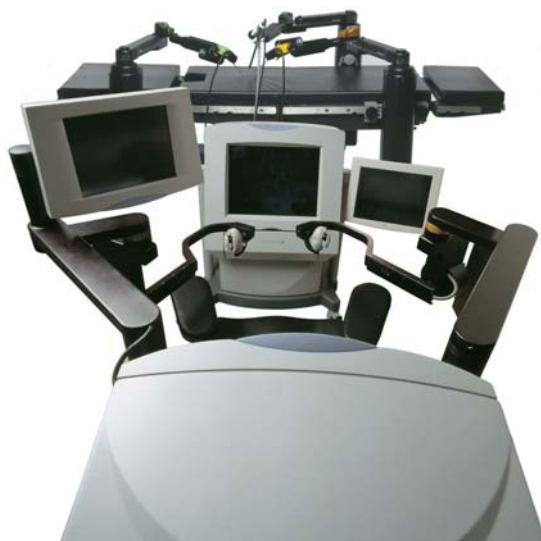
FIGURE 2.2. The Zeus® system, showing the patient side subsystem consisting of three robotic arms that are attached to the table. (Reprinted with kind permission from Intuitive Surgical, Inc. www.davinciprostatectomy.com/images/aesop_images.zip and www.davinciprostatectomy.com/images/zeus_images.zip by Alexis Morgan, Sunnyvale, CA, USA. January 2007.)
