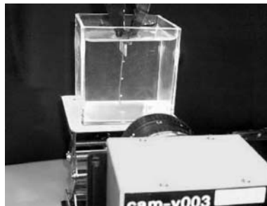
Figure 7.12. Camera head of vision system and artificial muscle
