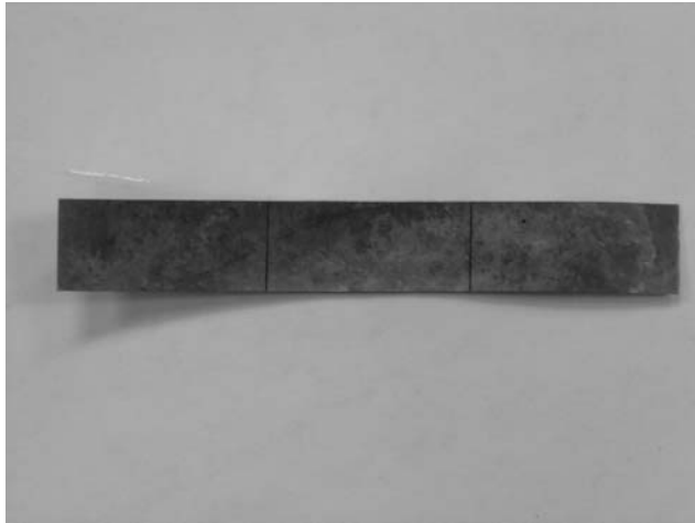
Figure 10.2. IPMC with three segment design
