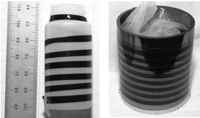
Figure 5.6. Synthesis of long films on a crucible. At right is the glassy carbon crucible employed to electrodeposit polypyrrole films up to a meter in length. The crucible is masked using Kapton ® tape, resulting in a film shown at left. Photos courtesy of Patrick Anquetil
