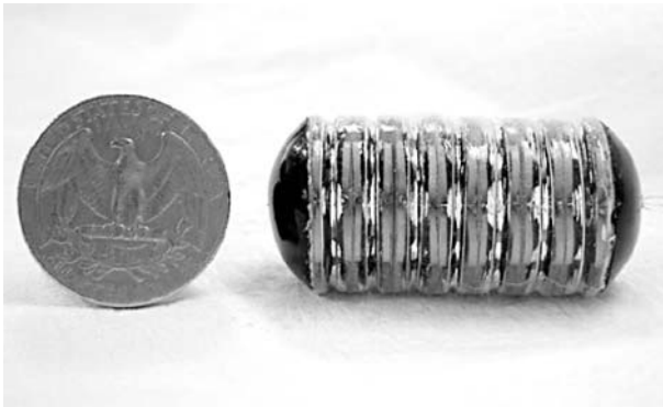
Figure 3.35. An inchworm robot
