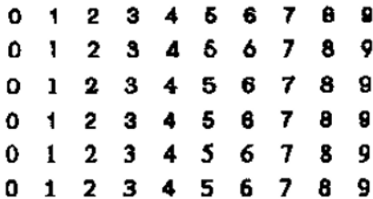
Fig. 9.1. Samples from machine-printed numeral database (originals printed at 6 pt, scanned at 300 dpi).
