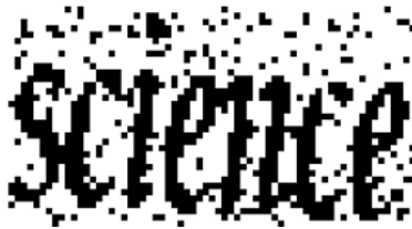
Fig. 15.5. Example of a PessimialPrint challenge: an English word is chosen at random, then the word (as a whole) is typeset using a randomly chosen typeface, and finally the word-image is degraded according to randomly selected parameters (with certain ranges) of the image degradation model.
