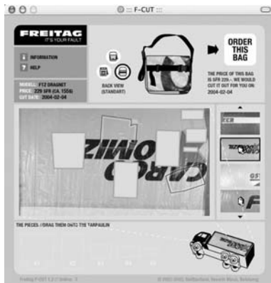
8.8 A much-praised computer tool for mass customisation. The Web interface allows customers to pick the material from a range of tarpaulins and make their own cutting patterns for their choice of bag. Image www.freitag.ch
