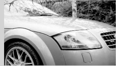
6 Car engines are designed to fit within the bonnet profile that is defined prior to a styling freeze
