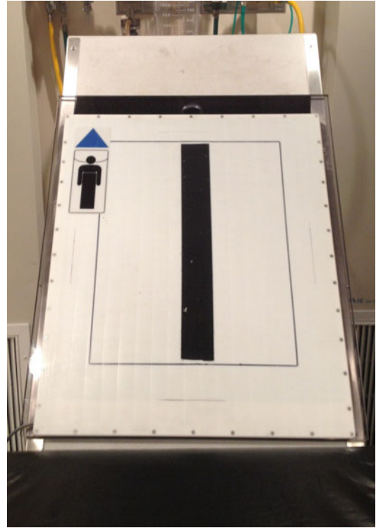
Fig. 6.1 Electromagnetic location board, placed at the head end of the table
