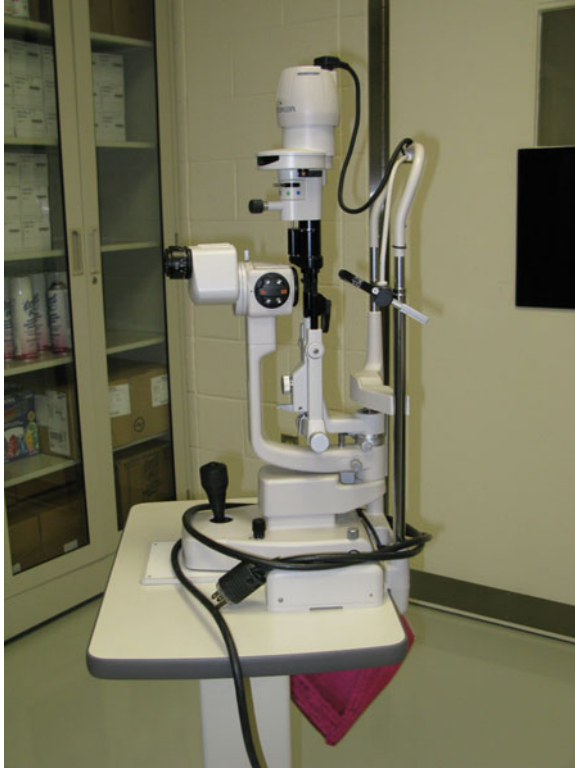
Fig. 2.1 A table-mounted slit-lamp biomicroscope offers excellent optics with multiple options for magnification and greater numbers of options for varying slit-beam width, height, and light color, and cameras may be added to the configuration to provide greater potential for stability and photographic documentation of lesions than camera options on handheld portable slit lamps
