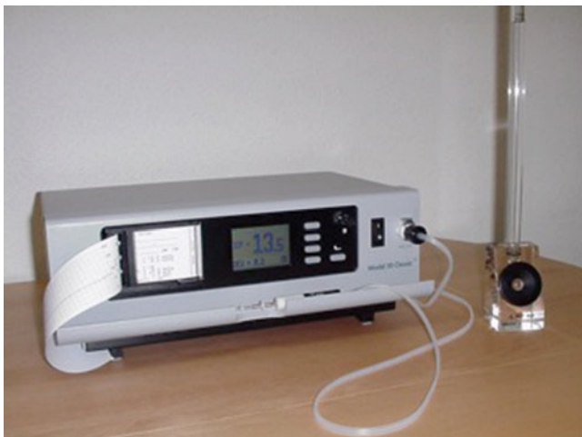
Fig. 2.23 The pneumotonograph is a tonometer that measures intraocular pressure by applanation of the cornea. Calibration is accomplished by placing the probe against a membrane in a manometer on the right , where the pressure is determined by the water level in the manometer. The intraocular pressure is recorded on the recording paper at the left side of the machine
