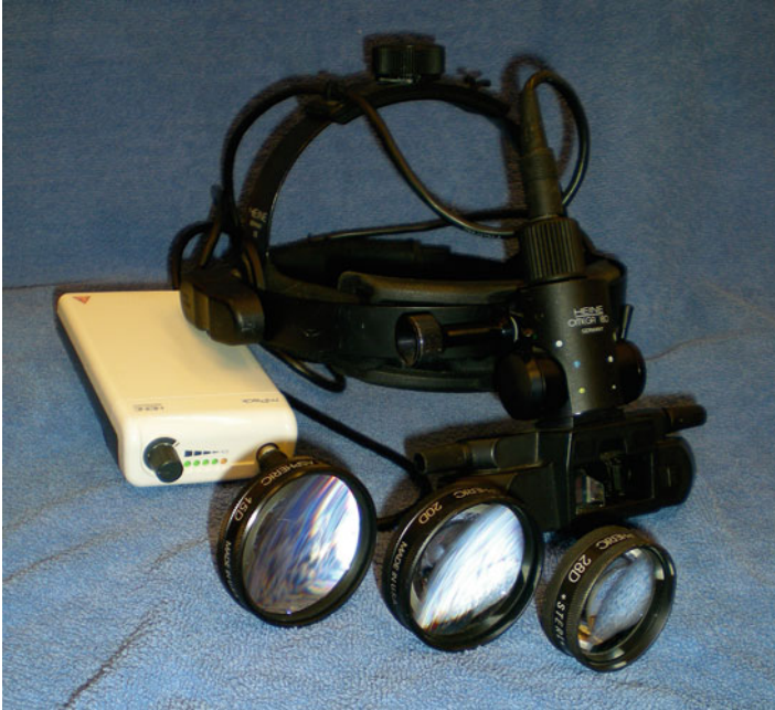
Fig. 2.10 The indirect ophthalmoscope with lenses of varying dioptric powers allows great flexibility for examining the ocular fundus with varying magnification. It is superior to the direct ophthalmoscope for evaluation of the fundus with respect to evaluating the greatest area of the fundus and assessing the overall appearance of the retina, choroid and optic disc
