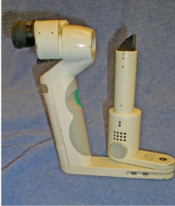
Fig. 2.2 The Kowa handheld slit lamp offers good optics and portability for the examination of eye in animals that are not sedated or that cannot be easily presented for examination by a table-mounted slit-lamp biomicroscope
