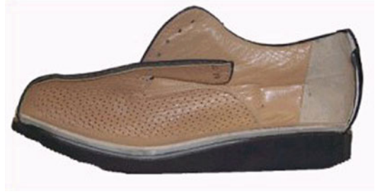
Fig. 26.4 Section of a shoe with “biomechanical properties”: the recessed heel allows a soft impact at heel strike; the point of rolling inserted immediately behind the metatarsal heads allows a smooth transition from midstance to propulsion; the presence a wider angle between the sole and the ground at the most anterior part of the shoe further reduces the stress at the level of metatarsal heads during propulsion and toe off
