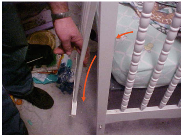
Fig. 9.11 Scene photograph of a crib in which a toddler was fatally hanged. Broken hardware on the bottom of the crib allowed the child to slip between the mattress and end of the crib (arrow), compressing his neck against the mattress
