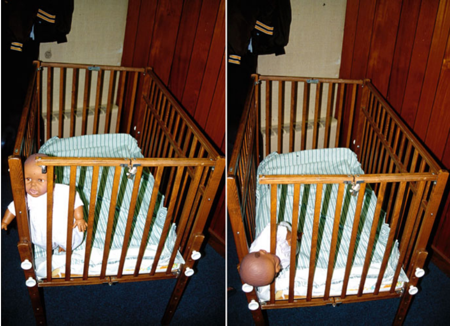
Fig. 9.12 Scene photographs (doll reenactment) demonstrating how an 11-month-old was fatally strangled in his crib. The bolt holding the corner of the crib together was missing
