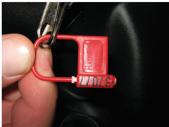
Fig. 7.6 Numbered plastic locks may be used to supplement chain-of-custody documentation
