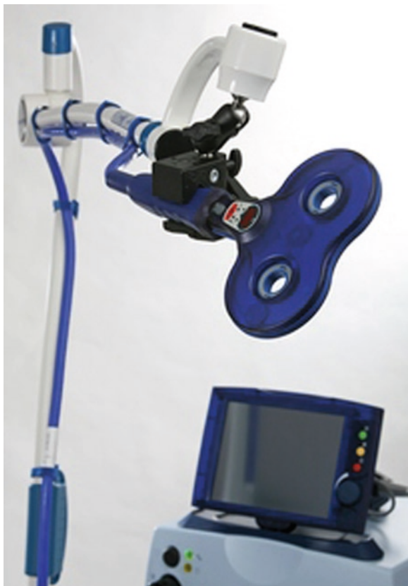
Fig. 88.2 The “figure of eight” coil consists of two overlapping loops of copper wire in a “figure of eight” arrangement. Current is induced under each of the two circular loops, but at the meeting point of the two loops the current sums up and is twice that beneath the edges of the two loops. Furthermore, this arrangement allows the stimulus to be more focal (1–2cm 2 ). Replicated by permission of The Magstim Company Ltd, Spring Gardens, Whitland, UK
