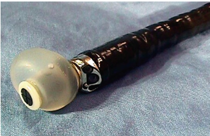
Fig. 3. A water filled balloon around the transducer of an echoendoscope helps to achieve acoustic coupling.
