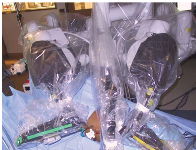
Fig. 6. Docking of the robotic cart. Note the space between the surgical arms.
