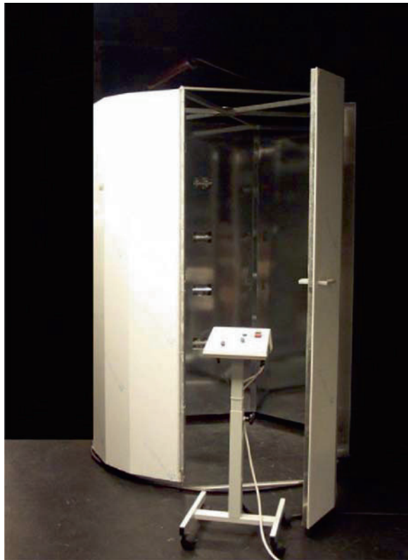
Fig. 1. Sun-simulating UV irradiation cabin (21).
