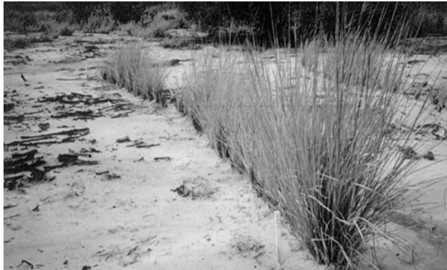
Fig. 8.9. Vetiver trials and old gold mine tailings. This old gold mine tailings site had a pH of 2.7, high in As (970 mg/kg), zinc, lead, and manganese. Very good growth was recorded 11 months after planting with adequate supply of lime (20 T/ha) and fertilizers.
