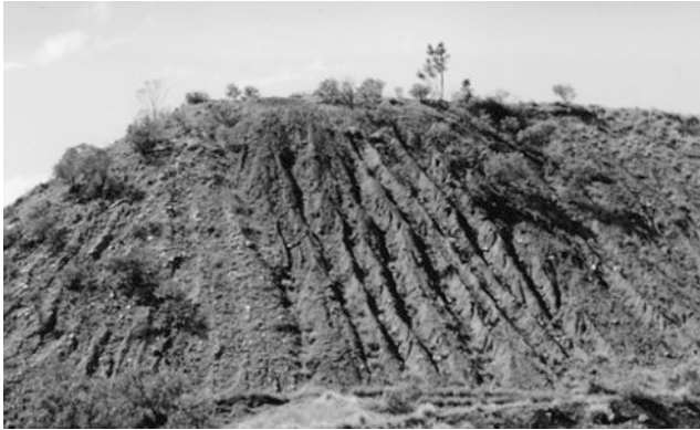
Fig. 8.10. Highly erodable coal mine overburden. This stockpile of coalmine overburden with 40^\circ slope is highly erodible. It is saline and sodic and remained mostly bare of vegetation in the last 30 years.
