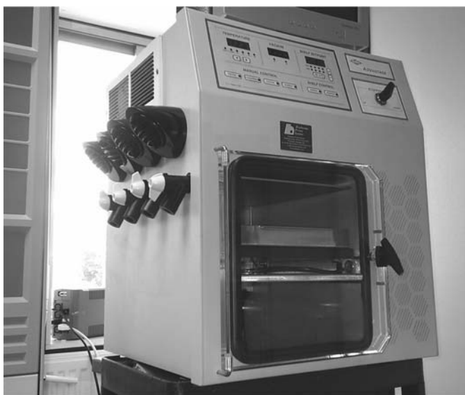
Fig.1. Typical benchtop freeze-dryer suitable for drying from flasks via the manifold or from trays of vials placed on the chamber shelf. (Photo Courtesy of Biopharma, UK.)
