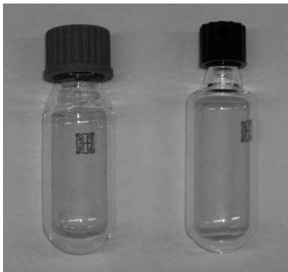
Fig. 1. Glass centrifuge tubes made by Ochs (Bovenden, Germany). To the left, a glass centrifuge tube used for aerobic strains. To the right, a centrifuge tube used for anaerobic strains. The narrow neck is sealed with a rubber stopper, which fits inside the screw cap, and has a hole in the top.
