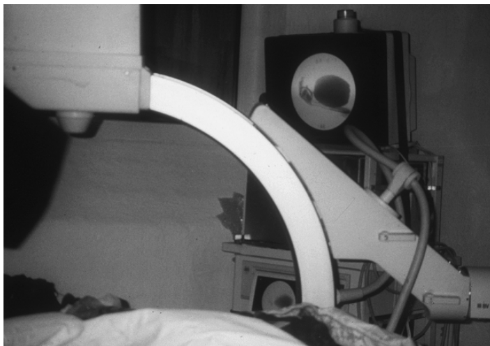
Fig. 8.12 The use of fluoroscopy for primary survey enables hazards to be identified and located. Fluoroscopy reveals the presence of a live grenade within the body bag (note image on screen in the background)
