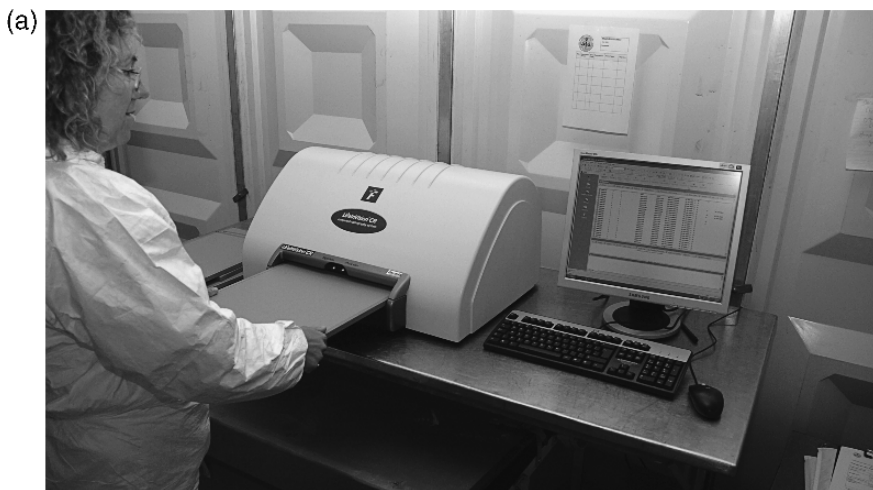
Fig. 8.6 Two options for digital radiography. (a) Computed radiography (CR) and (continued)
