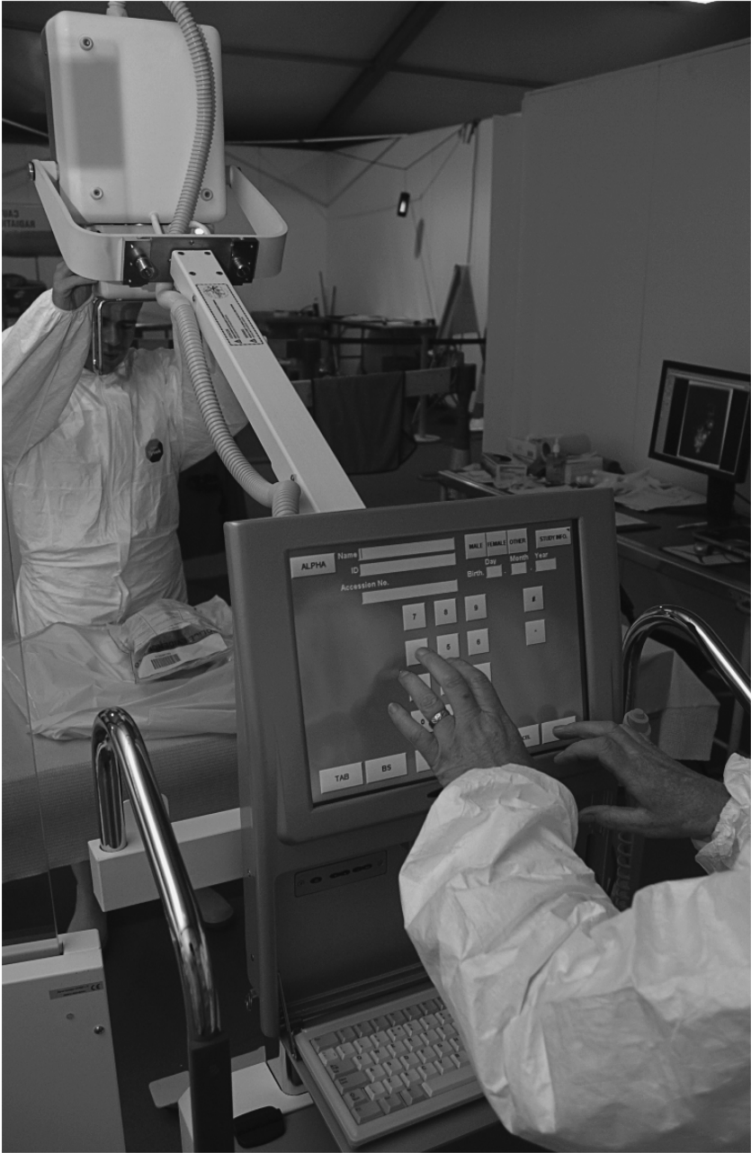
Fig. 8.6 (b) direct digital radiography (DR)
