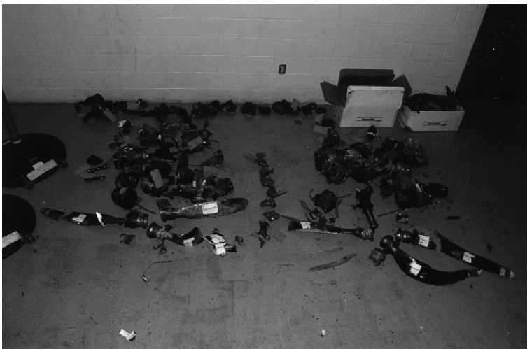
Fig. 3.6 Recovered airplane components laid out for reconstruction and again, demonstrating severe fragmentation (photo by Richard G. Marty Jr.)
