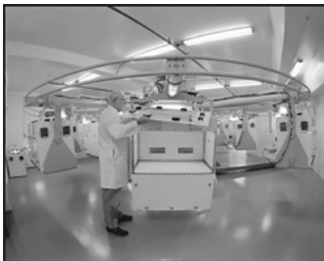
Figure 49-3. The 24-foot small animal centrifuge at the Center for Gravitational Biology Research (CGBR), NASA Ames Research Center, Moffett Field, CA. (Photo by Thomas Trouwer. Reprinted courtesy of NASA Ames Research Center.)
